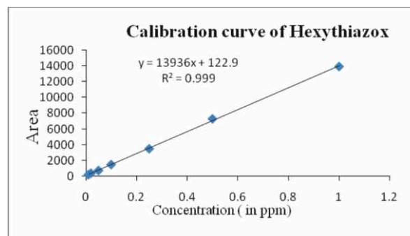
Fig. 2: Calibration curve of analytical standard of Hexythiazox in GC-ECD
