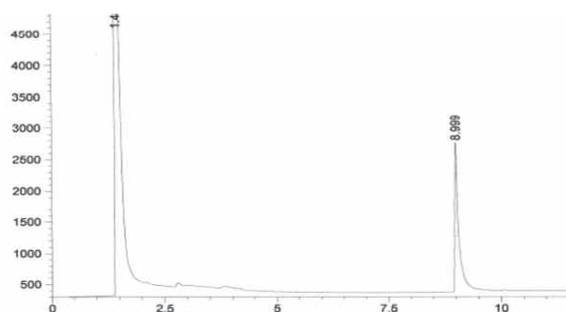
Fig. 3: GC-ECD chromatogram of 1 ppm standard Hexythiazox solution in ethyl acetate
